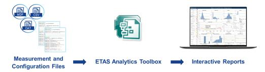
The data recorded and uploaded to some storage location on a server can be transferred to EATB. EATB provides a visualization of the relevant information and critical threshold violations.
